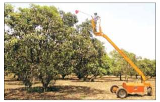
Self-propelled hydraulically hoisted platform for orchard management
